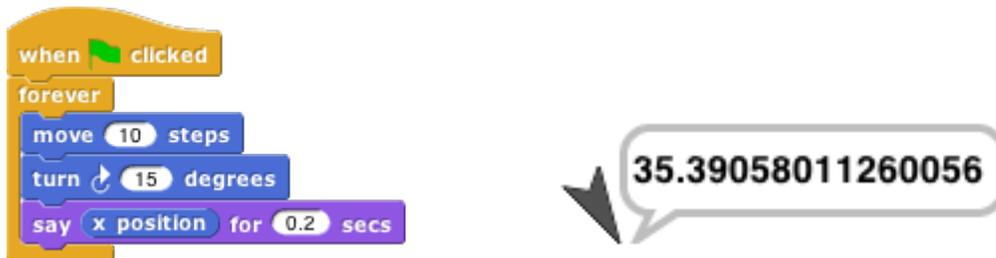
Here the `x position` reporter provides the first input to the `say` block. (The sprite's X position is its horizontal position, how far left (negative values) or right (positive values) it is compared to the center of the stage. Similarly, the Y position is measured vertically, in steps above (positive) or below (negative) the center.)
